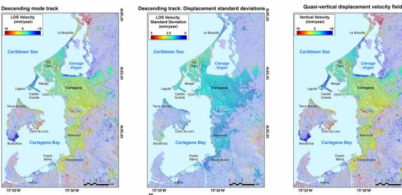
c) Time-series of LOS displacement of descending tracks data: Sentinel 1 and TerraSAR-X
