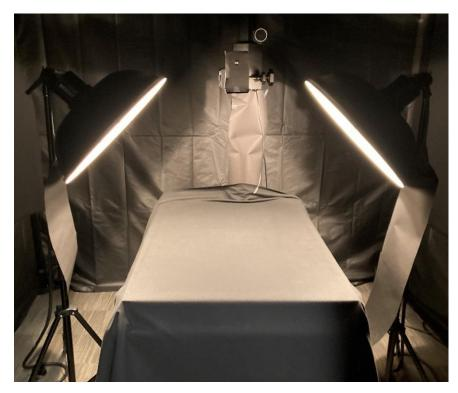
Figure 2: Copy stand setup with two modeling lights
