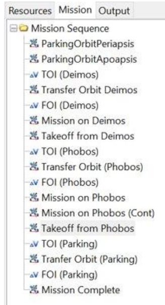
Figure 6. Option for the SCOTT Mission Profile for a single rover. Figure 6 shows the list of steps in the mission using General Mission Analysis Tool (GMAT).
