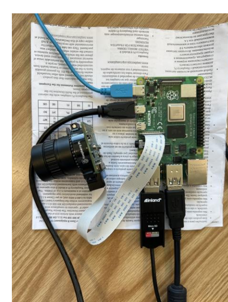
End to end connection with the mic, and camera on Raspberry Pi 4
