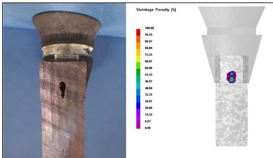
Fig. 5. Experimental shrinkage defect vs final simulation results
