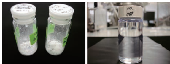
Figure 6. Photograph of synthesized complexes (left panel) and a scintillator cocktail consists of Zr(iprac)_4 2222mg, PPO 993mg and POPOP 10mg in 20mL anisole (right panel).
