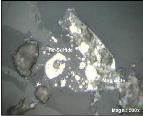
Fig 3: Complex intergrowth of iron-sulfides (pyrrhotite?), partly molten, and magnetite.
