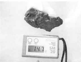
**Fig. 2.** One of ordinary chondrites found in Moulton Escarpment by KOREAMET. The bottom is magnetic susceptibility (MS) meter showing that the meteorite is relatively high in MS and probably H-group.
