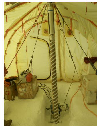
Fig 2 Ice drilling system
