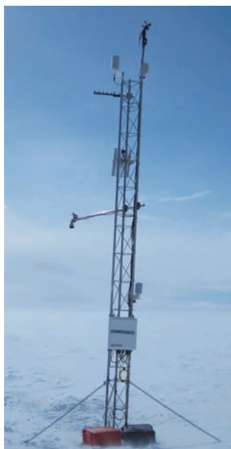
Fig. 1. Lorne AWS, consisting of two R.M. Young RTD and one Vaisala HMP 155- all three in Gill Radiation shields, LI200X pyranometer; SR50A ADG, and R.M. Young Wind Monitor system. Within the electronics enclosure is a Paroscientific pressure sensor.
