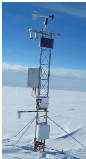
Fig. 2. Kominko-Slade station prior to servicing. Instrumentation consists of a Weed platinum resistance thermometer (PRT), a two-junction thermocouple temperature-difference sensor set (measuring temperature difference between the sensor boom at top of the tower and the half meter mark above the snow), an R.M. Young Wind Monitor, a Vaisala HMP 45 for humidity, and a Paroscientific pressure sensor within the enclosure.
