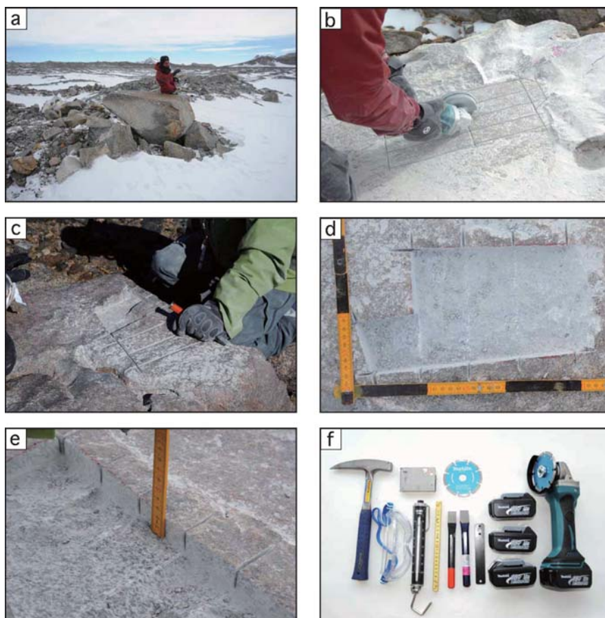
Fig. 1. Photographs of the sampling procedure for surface exposure dating. (a) Overview photograph of a boulder on a moraine. (b) the outline of the sample pit and cross cuts are made on the rock surface using a portable electric rock cutter. (c) Block samples are removed using a hammer and chisel. (d) Sample pit after cutting and block removal. (e) Measuring depth along the sharp edges of the sample pit made by the rock cutter. (f) The portable electric rock cutter, batteries, and other essential tools for this sampling technique. We used a rock cutter designed by the Makita Corporation (GA402DRF).
