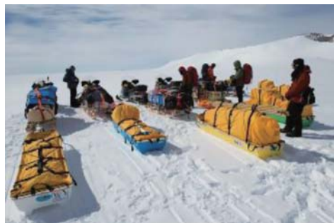
図 18 ナンセンソリと岩石輸送ソリの連結 Fig. 18. Connection between a Nansen sled and a cargo sled for transporting rock samples.
