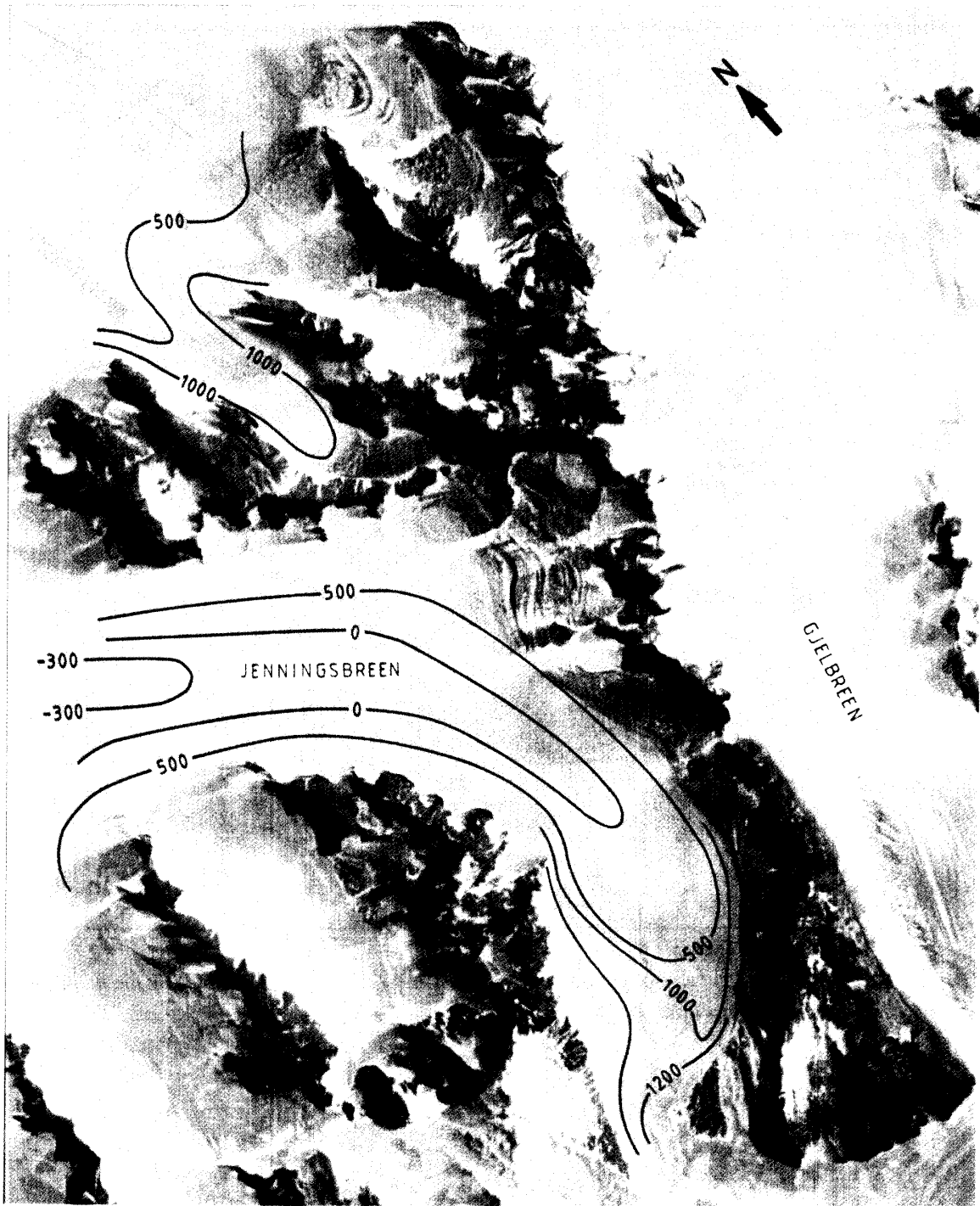
Fig. 4a. Landsat Thematic Mapper satellite image of Jenningsbreen and De Breuckbreen displaying subglacial bedrock contours in m.
