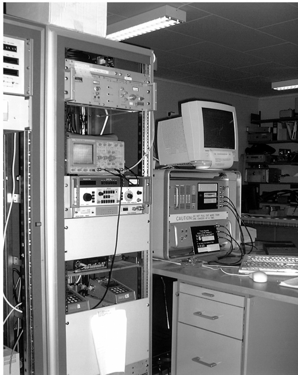
Fig. 7. The Lowell ionosonde. The Lowell unit itself is beneath the computer monitor. The rack to the left contains frequency reference equipment including synchronisation with nearby instruments (Photo: Bjørnar Hansen).
