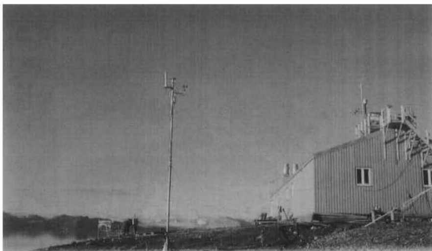
Fig. 2. Japanese Ny-Ålesund Observatory and our meteorological tower. Sensors for measuring temperature, humidity, wind speed, wind direction and solar radiation were mounted on the tower, and a sensor for atmospheric pressure was installed in the room of the observatory.
