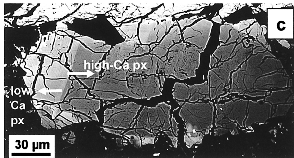
Fig. 4c. BSE image of Px 3 showing high-Ca core and low-Ca rim. Chemical zoning in the high-Ca pyroxene (from right to left) toward the boundary with low-Ca pyroxene is visible.
