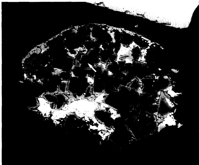
Fig. 2a. The spherule SS-4 is 125 \mu\text{m} in diameter and contains about 30 relict forsterite grains with zonal structure. The wight matrix surrounding the relict grains has composition of (\text{Fe}, \text{Ni})_{12}\text{S}_{13} .
