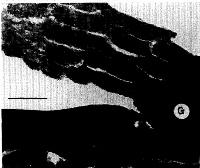
Fig. 12. Relationship among glass and alteration layer observed by TEM from ultramicrotomed thin-section-experiment 1 month in H_2SO_4 solution with pH1 conditions at 80^\circ C (G=glass; scale bar=400 nm).
