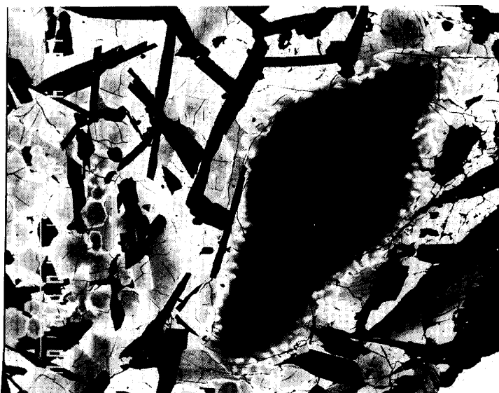
Fig. 7. Back-scattered image of a porphyritic olivine in Asuka-881371. Olivine shows Mg-rich core surrounded by a thin layer of an Fe-rich rim. Field of view is 1.5 mm.
