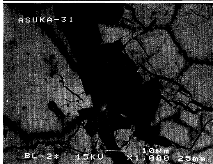
Fig. 4c. Back-scatter electron (BSE) image of sample A31-BL2: Plagioclase (dark gray) and K-rich phase X (gray) from a small inclusion in a large fayalite grain.
