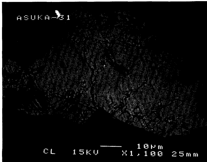
Fig. 2a. Back-scatter electron (BSE) image of sample A31-CL: Ca-rich pyroxene with lamellae, attached to a large plagioclase fragment (gray).
