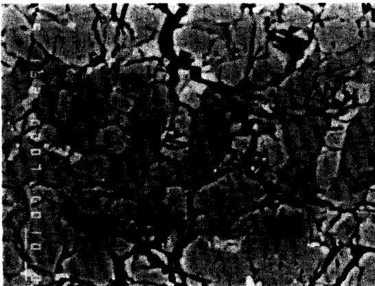
Fig. 17b. BSE image of No. 161. Note a ladder structure consisting of diopside (Di) and silica mineral (Si). Width is 56 \mu m.
