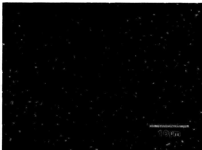
Fig. 10. A region of matrix having a high density of Fe-Ni-rich particles (backscattered SEM image).
