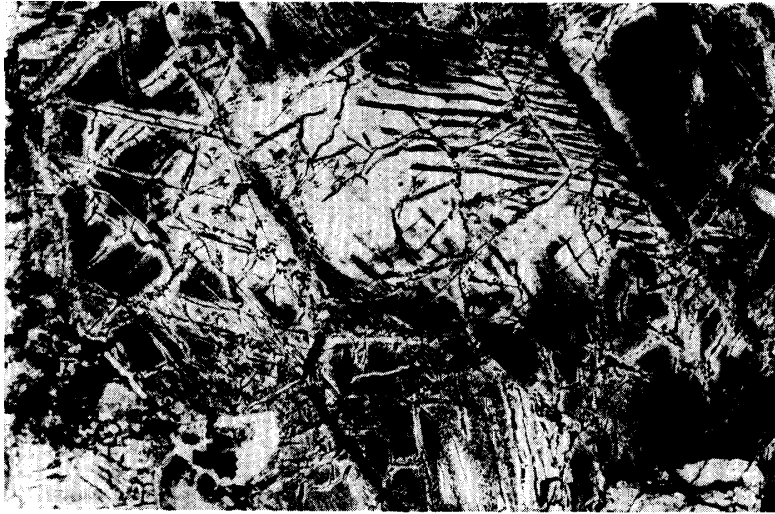
a. Olivine crystals with numerous inclusions of fine metal particles. Open.
