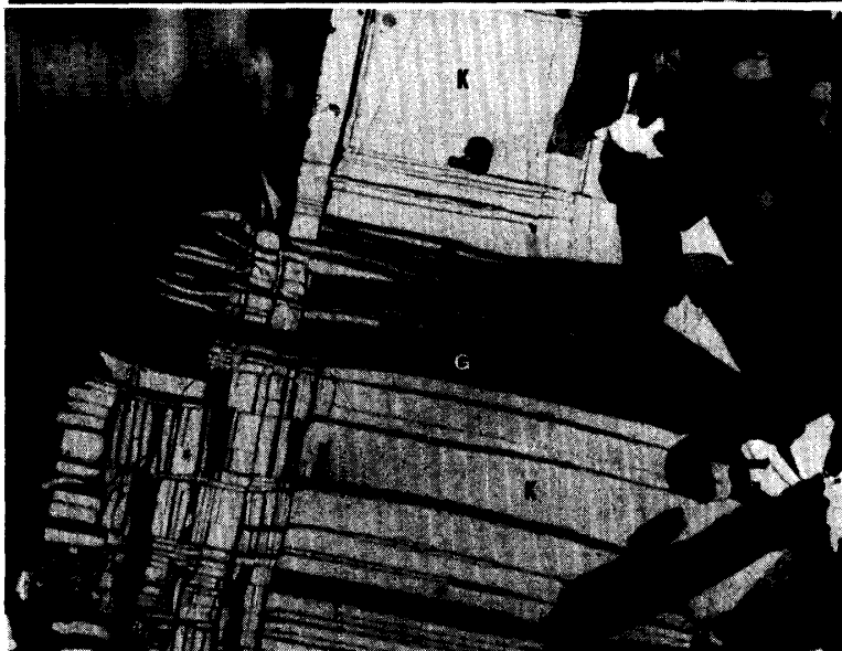
Fig. 8. Well oriented graphite lamellae (G) in kamacite (K) in St. Marks meteorite. Graphite also contains fine kamacite lamellae.
