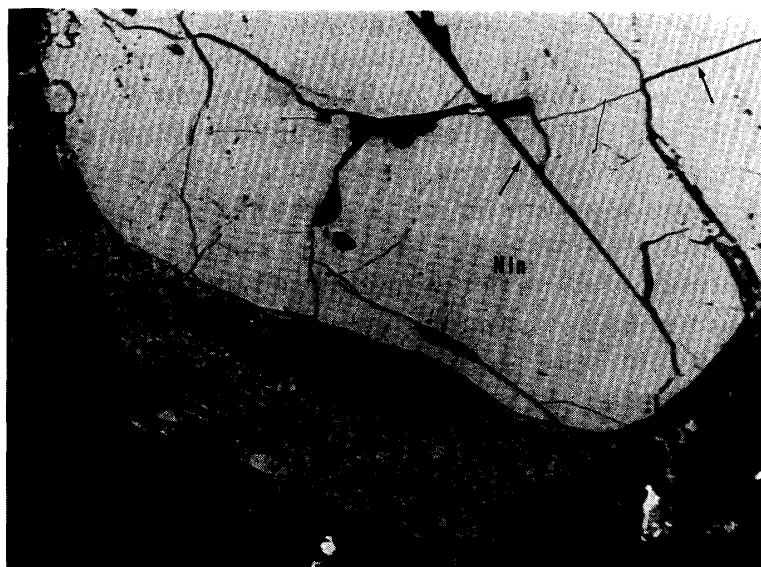
Fig. 2. A detail of a niningerite-oldhamite clast from Qingzhen. Rounded grain of niningerite (Nin) with well developed cleavage along (111) directions (arrows). The grain is covered with a djerfisherite grain (Djr) with advanced Qingzhen Reaction. Length of photograph 300 microns.
