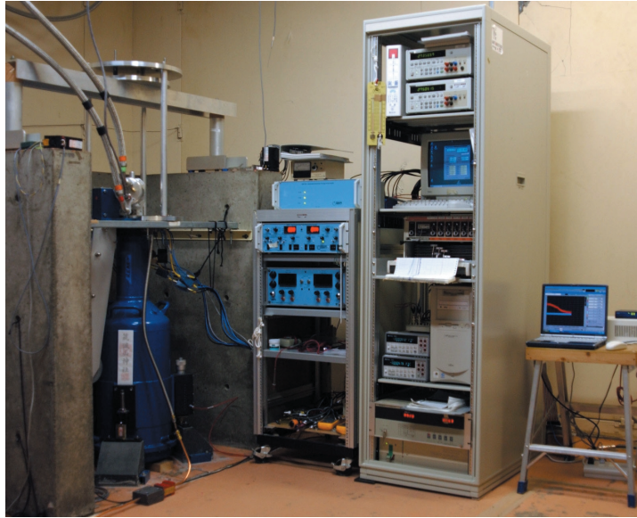
Fig. 5. A new superconducting gravimeter CT(#043) was placed to the pillar site for routine operation.
