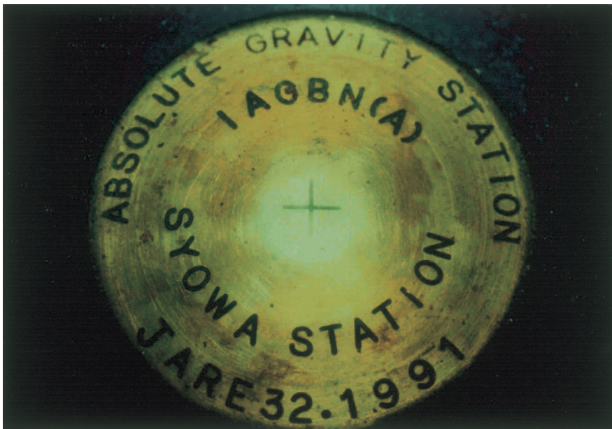
Fig. 6. (Top): Sketch of the gravity observation hut, where the marble plate within the concrete base for AG measurements is installed. The SG TT70 (#016) is hung from the pillar at the northeast corner. (Bottom): The brass disk buried in the marble plate indicates the Syowa IAGBN(A) 0417 marker.
