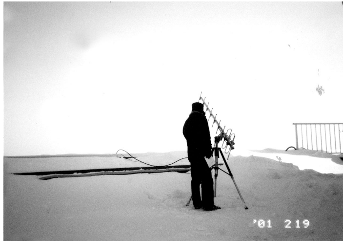
Fig. 4. Tracking the ECC ozonesonde using a YAGI antenna on the roof of a building in Wakkanai.
