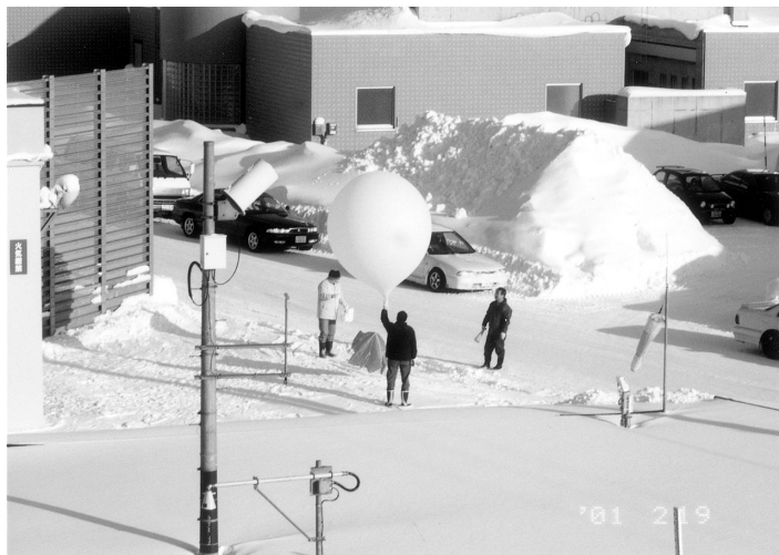
Fig. 3. The release of an ECC ozonesonde at Wakkanai.
