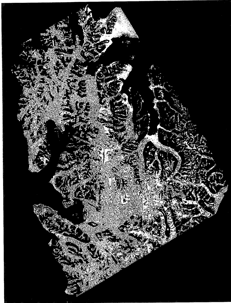
Fig. 2. Differential interferogramme over northwestern Spitsbergen from ERS-1 data recorded on ascending orbits the 17 and the 23 September 1991 (six days interval). The image is oriented to the North and covers the area of one complete ERS-1 scene (100 × 120 km). Despite of the scale, clear fringes are visible on several glaciers on the eastern part of the image while due to the meteorological condition the western part is characterised by a low coherence and lack of fringes. Inverse conditions as well as radar features were observed between the 23 September and the 3 October and on the nine days interval interferogramme not presented here.
