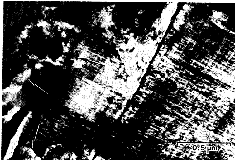
Fig. 3. TEM micrograph of the boundary region between a carbonate grain (Mn-rich dolomite) and the phyllosilicate groundmass (upper left). Arrows indicate the contact. The apparent sharp "edge" is a cleavage plane in the dolomite, which had composition MgO 36.7, CaO 54.0, MnO 3.2, FeO 6.1 wt%.
