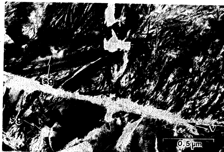
Fig. 4. TEM micrograph showing various phyllosilicate growth morphologies within a chondrule-like object, which exhibits a thin vein (arrow v) filled with amorphous material. Chrysotile grains with sectorial growth morphologies (arrows Sg) are common, but acicular forms predominate, here in very fine-grained form.
