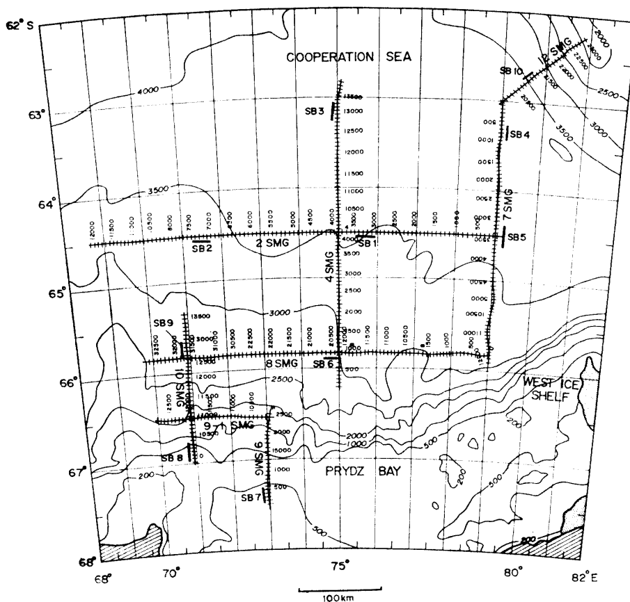
Fig. 5. Lines of seismic reflection survey and sites of sonobuoy seismic refraction survey off the Amery Ice Shelf. SB: Sonobuoy.
