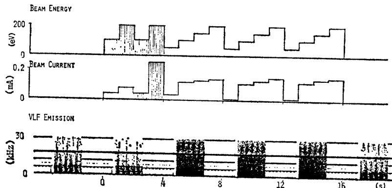
Fig. 6. VLF ionogram in K-10-12 experiment. Emissions with broad frequency spectrum are observed. Intensity is modulated by a spin motion.
