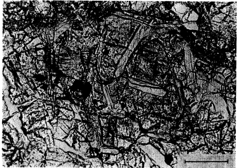
Fig. 6. An ophitic-textured fragment composed of pigeonite and plagioclase in Yamato-7308. The bar is 0.1 mm in length.
