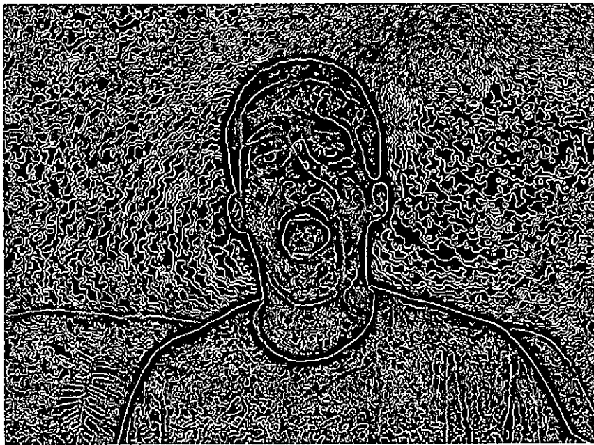
Fig. 3.3: A poor quality edged image by applying the OpenCV Canny edge detector function with a low threshold value of 0 and high threshold value of 0 to an web cam image.
