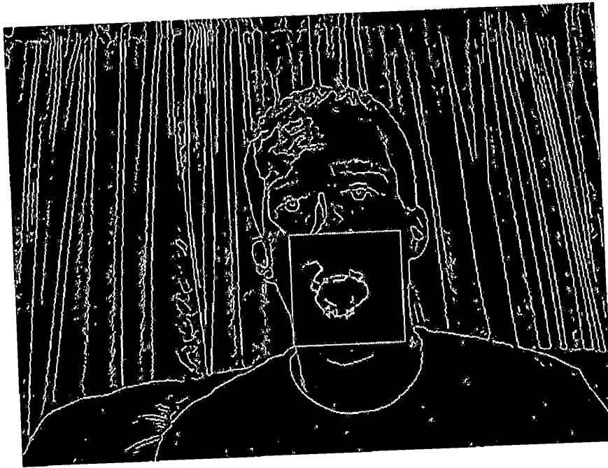
Fig. 5.10: Result of using the GapFiller function with gap filling pixel size parameter of three pixels and FindLargestEdge function.
