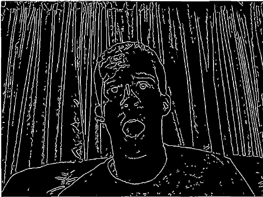
Fig. 3.2: The result of applying the OpenCV Canny edge detector function with a low threshold value of 20 and high threshold value of 20 to an input image.
