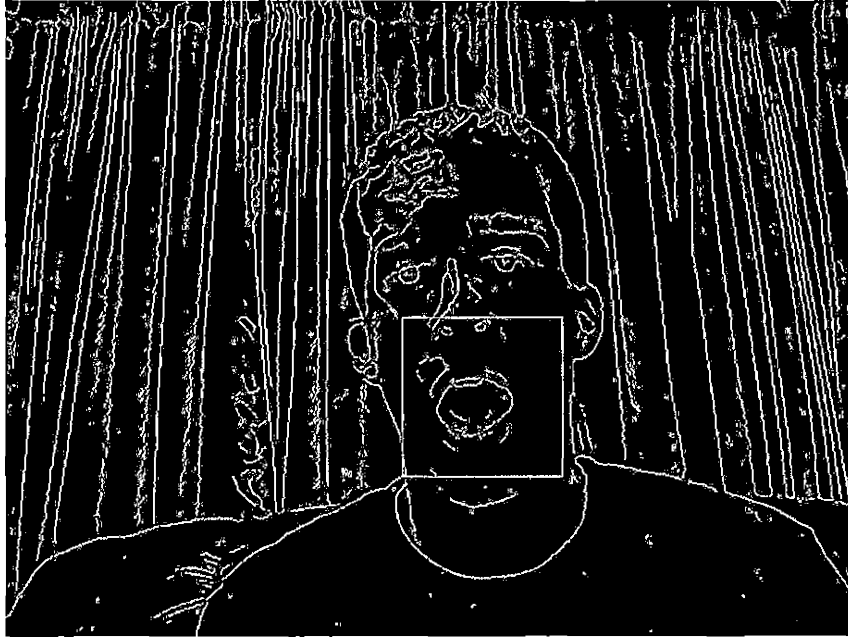
Fig. 5.7: Example of an edged input image that is used by the system.
