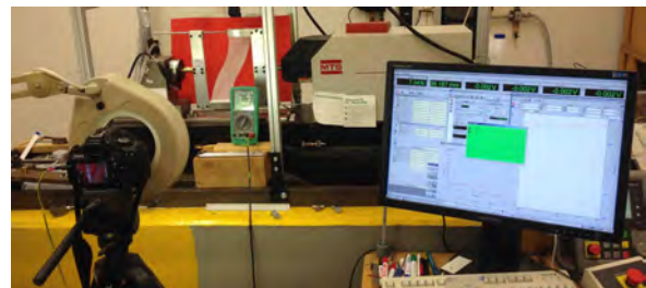
FIGURE 4. Experimental setup during shear deformation: Camera and illumination devices on the left, pantographic sample mounted in an MTS Tytron 250 testing machine in the middle, interface of control software on the right.
