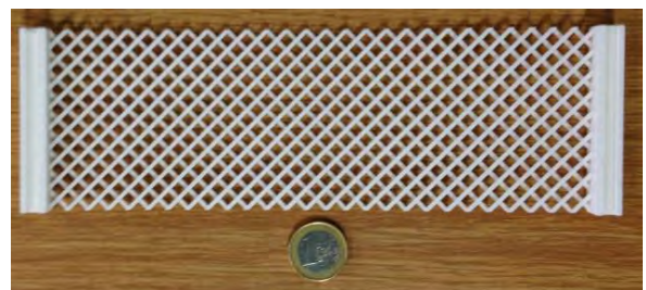
FIGURE 1. Example of a pantographic structure developed by [2].
