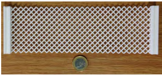
Figure 1: Polyamide sample of a PS developed by (dell'Isola et al., 2015b).
