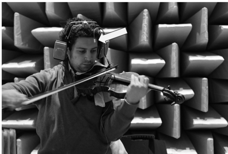
Figure 1. Violinist playing in a simulated concert hall, wearing extra-aural headphones with the recording microphone (marked by the arrow) attached to his instrument.
