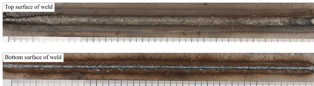
Figure 9. The top surface and the root of the hybrid laser arc welded joint with electromagnetic weld pool support technique using 17.7 kW laser power and 9.8 kW arc power at a welding speed of 1.3 \text{ m min}^{-1} .
