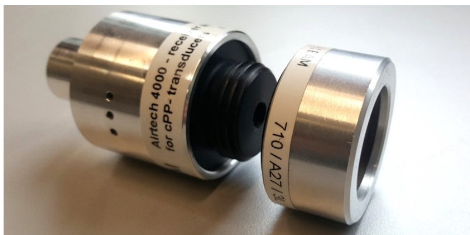
Figure 3.22: Cellular PP receiver for air coupled ultrasonic measurements. The receiver consists of the cellular PP transducer (right) and a preamplifier (left).
