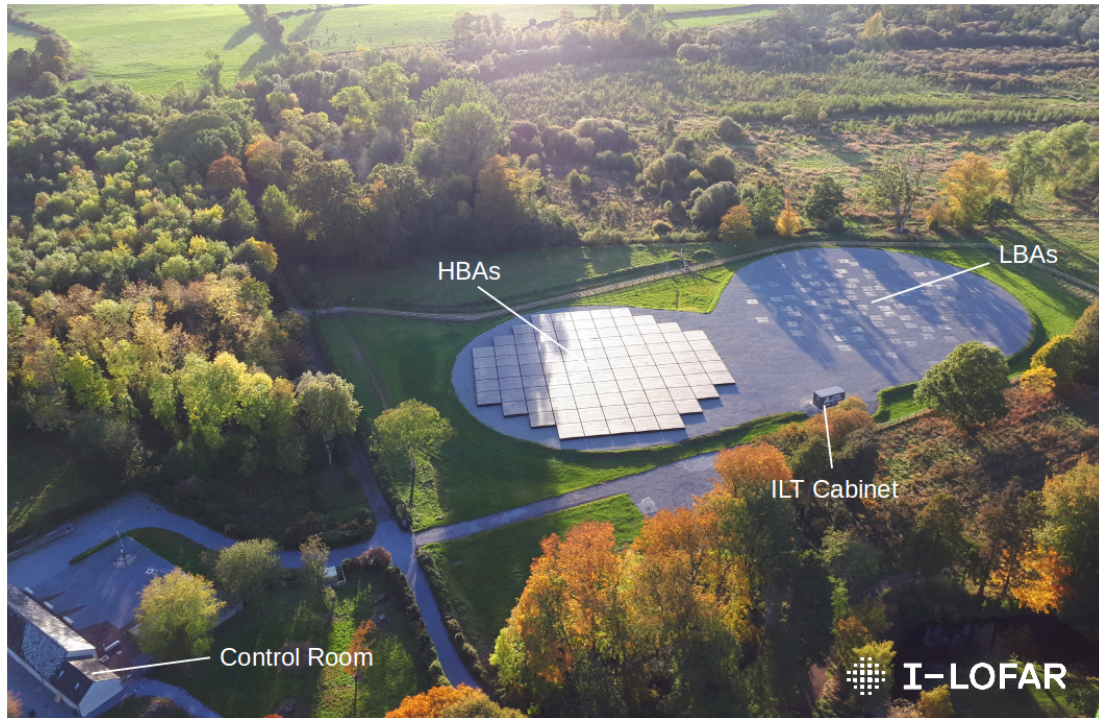
Fig. 1. Aerial photograph of the Irish Low Frequency Array station IE613 (I-LOFAR) at Birr Castle, County Offaly. Data from the LBAs and HBAs are transferred to the ILT Cabinet (centre right) via coaxial cables where they are amplified, filtered and digitised. In international mode, data are transported to Groningen in the Netherlands at \sim 3.2 Gbps. In local mode, data are processed using REALTA in the I-LOFAR Control Room (bottom left). Image credit: Alison Delaney (Birr Castle).
