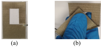
Fig. 2: Fabricated antenna prototype: (a) Top view. (b) Folded antenna demonstrating its flexibility.
