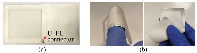
Fig. 2. (a) Screen-printed antenna prototype upon U. FL connector assembly. (b) Antenna under deformation demonstrating its flexibility.
