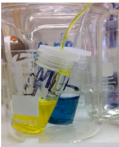
Figure 4. Reactant vials containing methyl 2-diazo-2-chlorophenylacetate ( 9 ) (yellow) and \text{Rh}_2(\text{OAc})_4 (blue).
