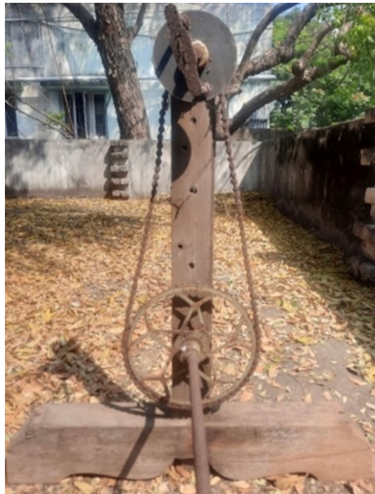
Figure 11 – Second model of the copper wound machine (side view). Photo courtesy: T.N. Sambasivan.
