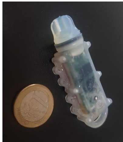
Figure 30 - Final embedded system for seaweed monitoring encapsulated.
