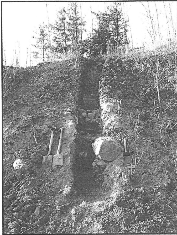
Figure 1.9 The completed trench at Strawberry Creek, about 3m deep. Note the transition from fine-grained sediments at the top to till material towards the bottom.
