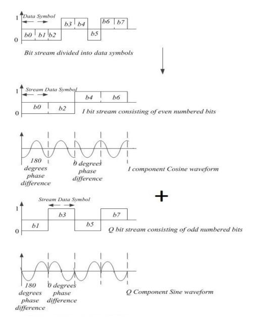
Figure 2.1: Formation of I and Q Components in QPSK
