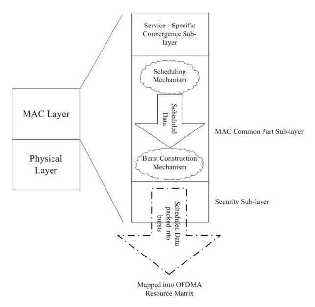
Figure 3.1: Relationship between Scheduler and Burst Construction Mechanism
