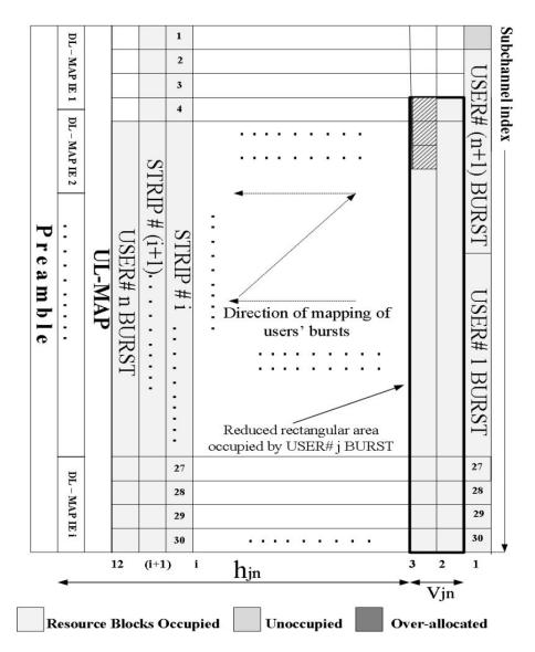
Figure 4.7: Rectangular area after moving resource blocks in BCFP
