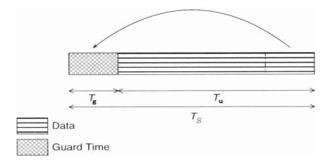
Figure 2.8: Basic Structure of OFDMA time symbol [29]
