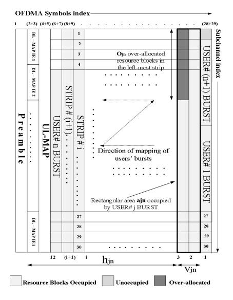
Figure 4.5: Over-allocation of resource blocks in a burst
