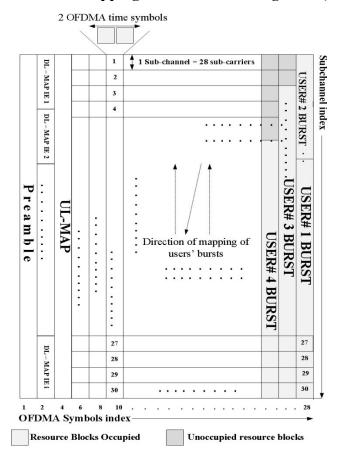
Figure 3.4: Mapping of users' burst to resource matrix in eOCSA
