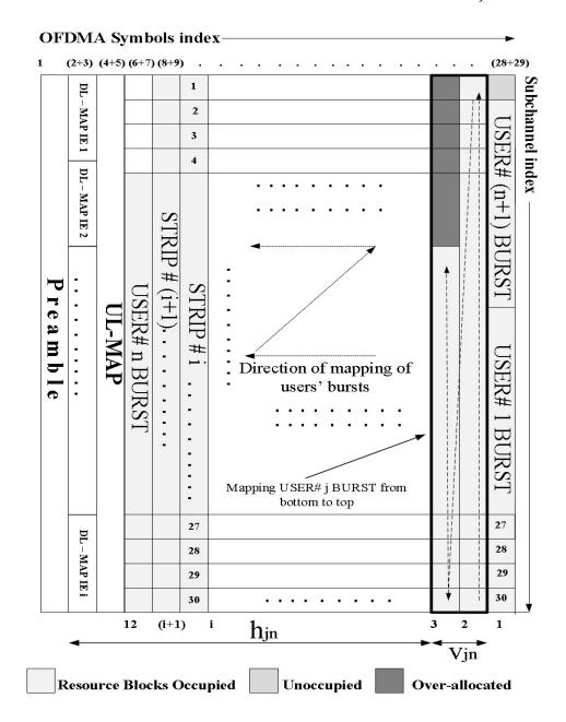
Figure 4.4: Burst mapping in BCFP Algorithm
