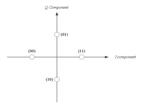
Figure 2.3: Transition states of a data symbol in QPSK Constellation
