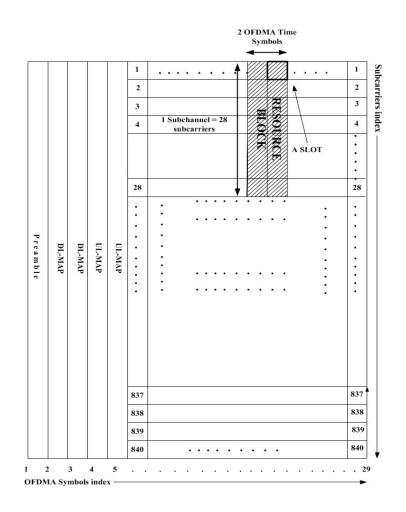
Figure 2.10: Structure of Resource Block in DL sub-frame
