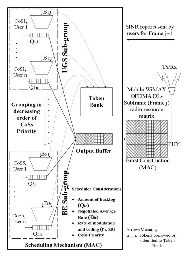
Figure 4.1: System Architecture at MAC Layer of Mobile WiMAX
