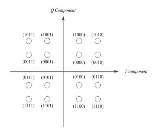
Figure 2.4: Transition states of a data symbol in 16-ary QAM constellation
