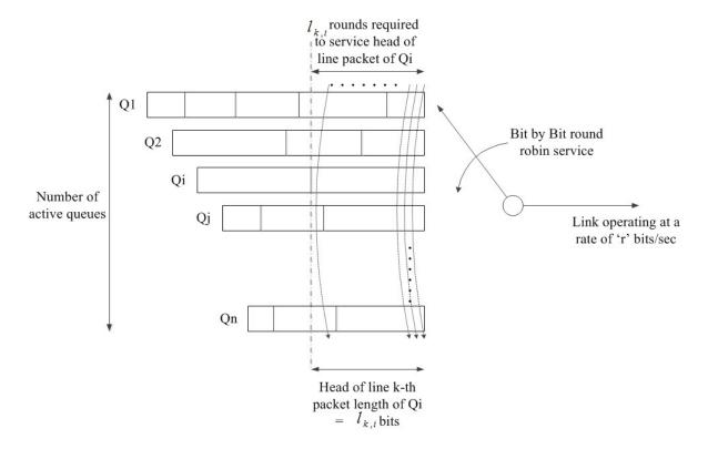
Figure 3.2: Practical bit by bit round robin system to approximate GPS system
