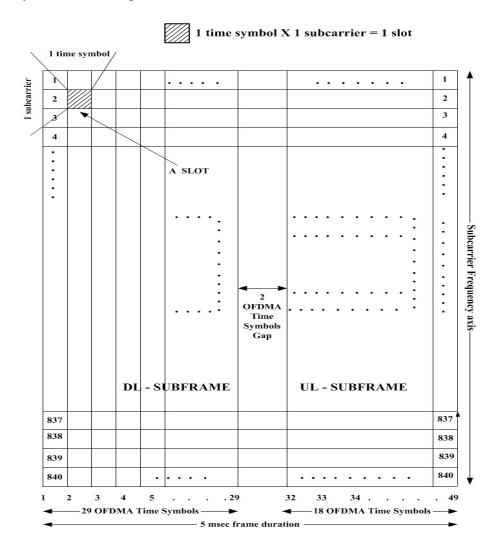
Figure 2.9: Mobile WiMAX frame showing DL and UL sub-frame
