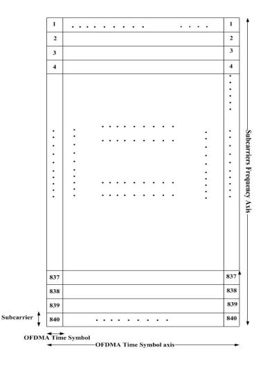
Figure 2.7: Time symbols and Subcarriers in Mobile WiMAX frame
