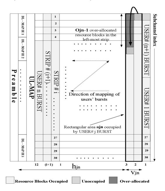
Figure 4.6: Moving resource blocks to the left-most strip in BCFP
