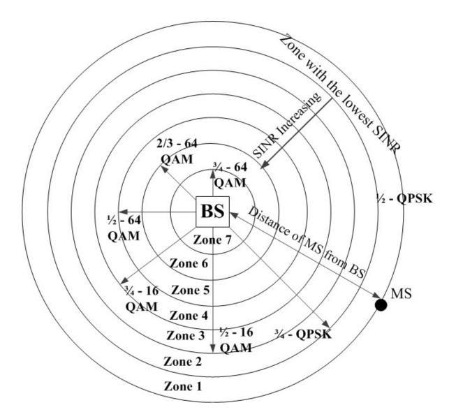
Figure 2.11: Classification of coverage area of a cell into different zones
