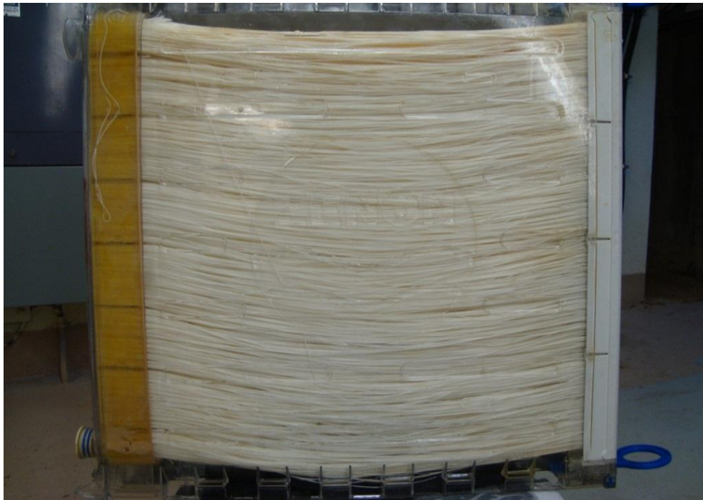
Figure 2-2: Membrane module used in this project (Bare point Water Treatment Plant- pilot plant)
