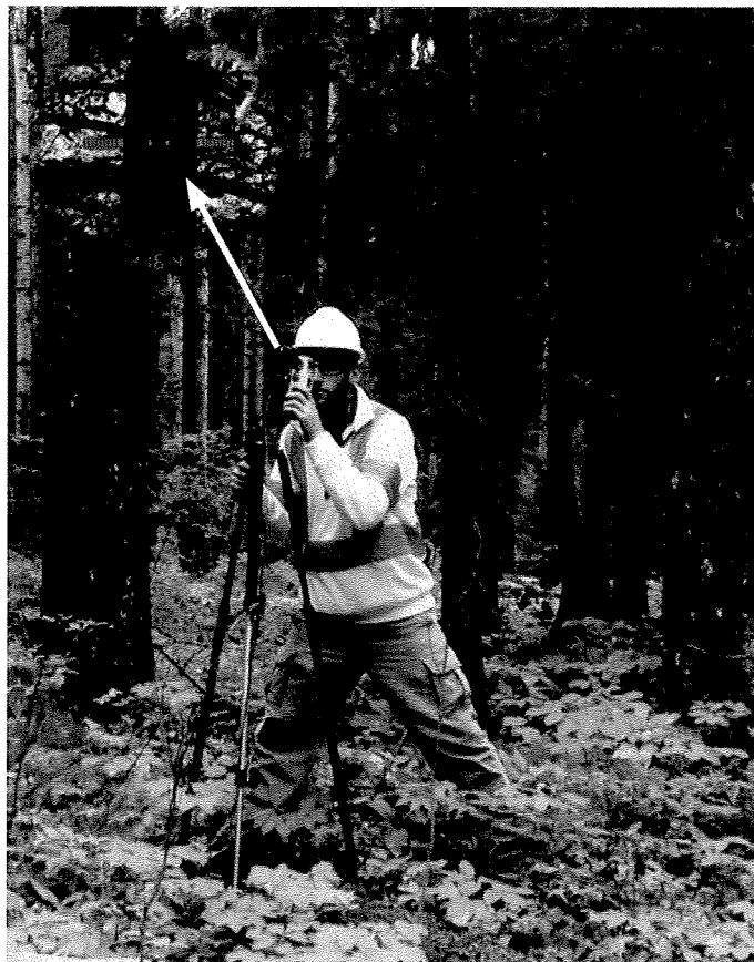
Figure 7. Criterion RD1000 electronic relascope being used to record stem profile data.
