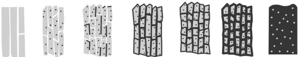
Figure 4.16 – Stages of the microstructures of Al-Ti-O-N coatings at increasing O concentrations.
