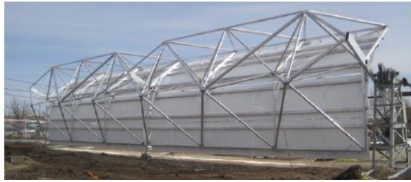
Figure 9-3 Abengoa Phoenix Gen 2.0 Collector
