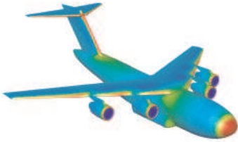
Figure 16: Numerical approximation of the pressure distribution on the surface of an aircraft.
